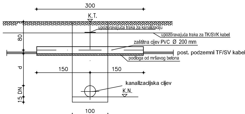
BEZ ZAŠTITNE CIJEVI ZA KABEL:
