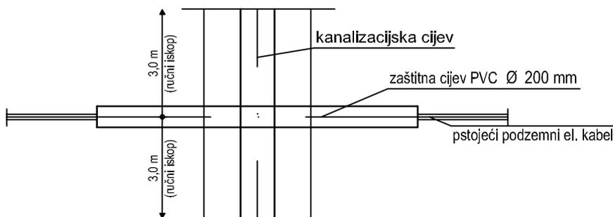
2. PARALELNO VOĐENJE ENERGETSKOG KABELA I KANALIZACIJE
