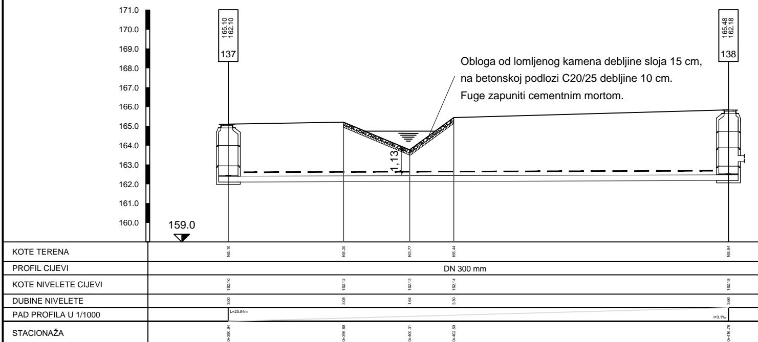
NACRT: DETALJI KRIŽANJA KOLEKTORA K 1-2 (OD STAC. 0+369.89 DO 0+402.59) I TLAČNOG VODA TV CS SP1 S VODOTOKOM
